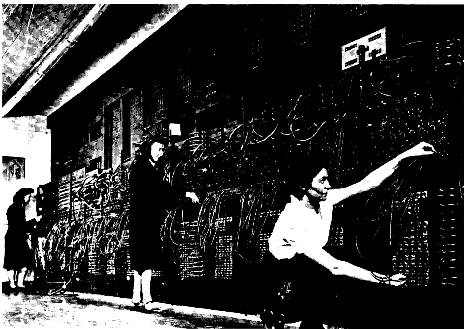
The ENIAC in operation at the University of Pennsylvania. This first large-scale electronic computer was tested in 1945 with the "Los Alamos problem," calculations important to the design of thermonuclear weapons. The lower photograph shows how the ENIAC was programmed by interconnecting the electron tube registers with cables inserted in plug boards.
